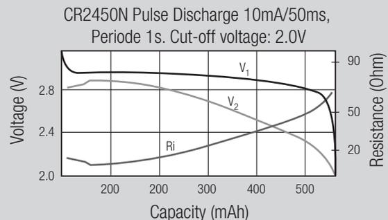
Figure 2: Pulse-current discharge characteristics<sup>1</sup> of the CR2450N cell.
