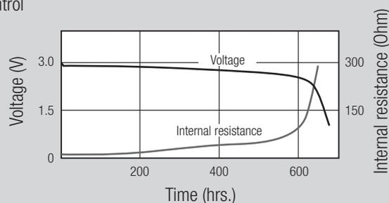
**Figure 1** Characteristic curve<sup>1</sup> of a CR2450N cell. Discharge load:  $R_1=3.32$  kOhm. Measurement of internal resistance during discharge: by applying the load  $R_2=150$  Ohm for 1s, every 3 hrs.
