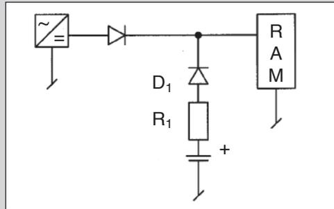
R<sub>1</sub> limits the recharging current when D<sub>1</sub> fails.
