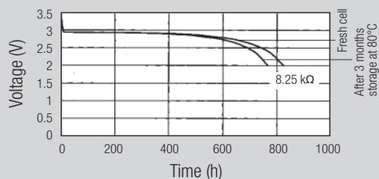
consequence, the ability of the cell to deliver high power is reduced. Especially when designing an application with high power demand (high current consumption, like pulse-loads), this factor must be carefully taken into account.
