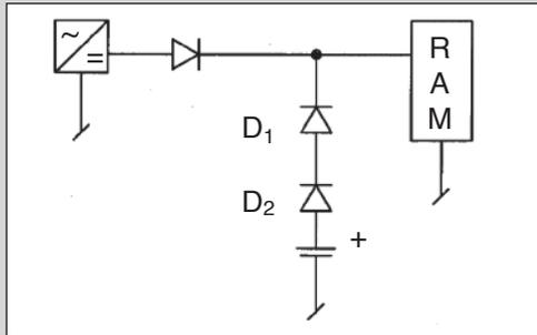
When D<sub>1</sub> is shorted D<sub>2</sub> still protects battery against recharging.
